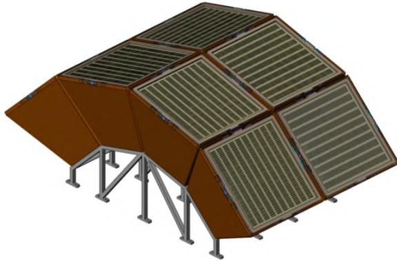
LOFT WFM Collimator, Mask & Detector Tray
